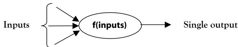
Figure 1 illustrates three inputs to the neuron. In practice there can be as many inputs as are required. Regardless of the number of inputs, there is just one output. The final model considered 30 such inputs, but only one output. To make a brain, many neurons are tied together as shown in Figure 2, which is an example of a four-neuron brain.
